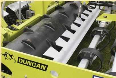
Water fillable drum roller with hardened steel blades for aerating the root zone.
