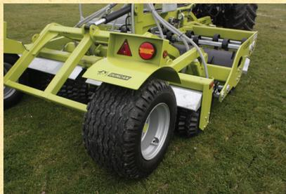
Wide profile flotation tyres on heavy duty hubs and stubs along with mudguards and LED lights.
