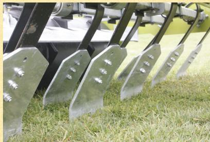
Individually sprung levelling boards for scratching the surface.
