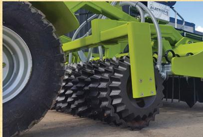
The finishing tool consists of cast prismatic roller rings.
