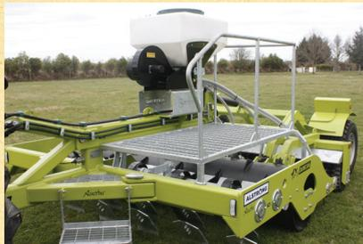
Large easy to access platform with safety rails for loading the seed hopper.
