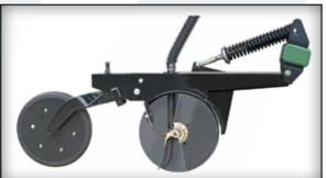
Great Plains 00 Series Openers are designed for min-till fluted feed drills. The OO Opener eatures 13.5" (34cm), 4mm blades mounted on 205 triple-lip sealed bearings. The 00 Opener has a 1/4" (19mm) lead opener blade. A rear depth-controlling press wheel uses a T-handle adjuster to provide 18 depth settings.
