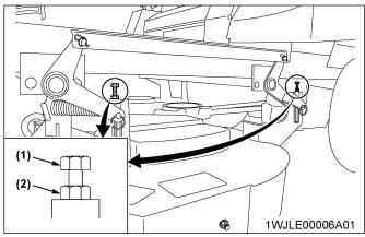
(1) Cutting height fine tuning bolt(2) Jam nut
