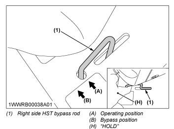
3. After moving, place both the right side and left side HST bypass rod back into the *"OPERATING POSITION"* hole.
